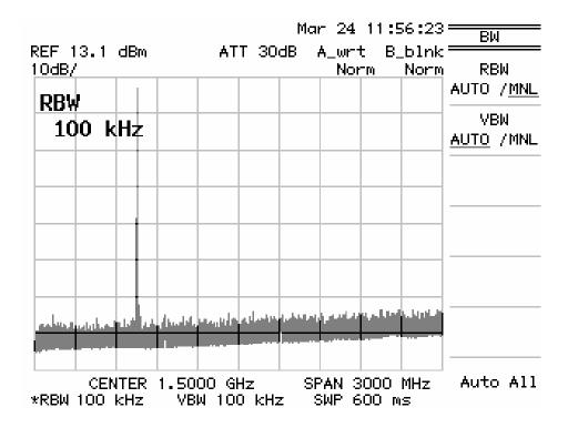
Both photographs indicate the fundamental frequency at 753 MHz. The values indicate that the required performance of -60 dB is met.
