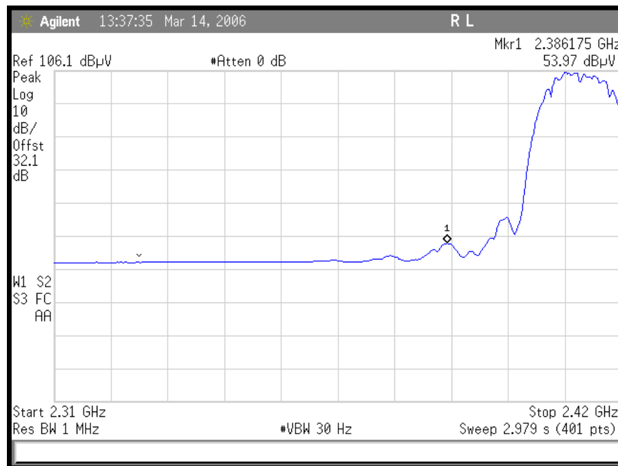
Plot 2. 802.11/b radiated restricted band 2310 - 2390 MHz Average
