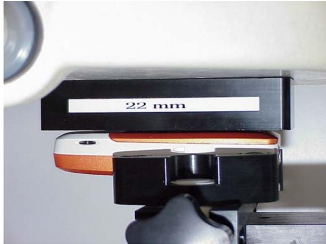
PPIRH-50 with 22 mm distance spacer before measurements
