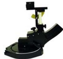
Device holder was provided by SPEAG together with DASY3.
