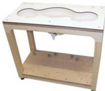
mounted usage at the flat phantom region. Reference markings on the phantom allow the complete setup of all predefined phantom positions and measurement grids by manually teaching three points in the robot.
