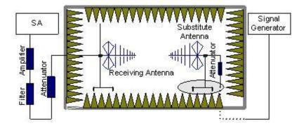
In the chamber, an substitution antenna for the frequency band of interest is placed at the reference point of the chamber. An RF Signal source for the frequency band of interest is connected to the substitution antenna with a cable that has been constructed to not interfere
