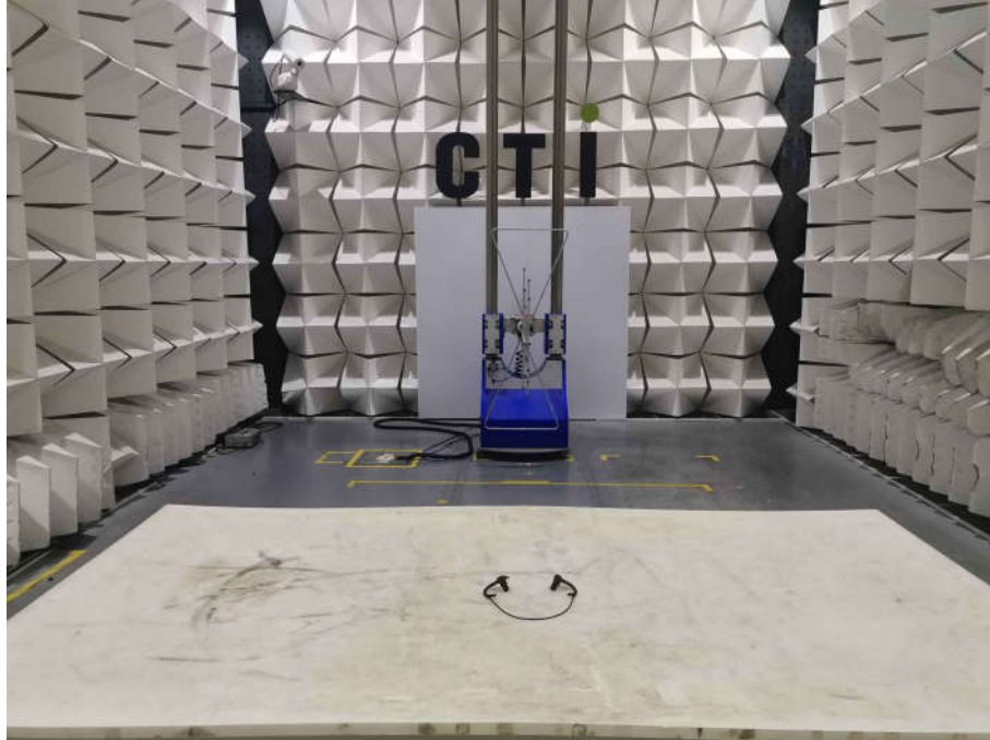
Radiated spurious emission Test Setup-1(Below 1GHz)
