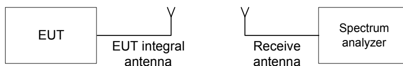
Figure 7.3.1 Emission mask test setup
