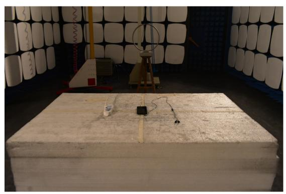
3. Radiated emission (9KHz-30MHz)
