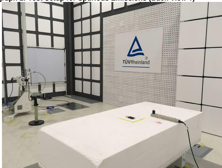
Photograph 2: Test Setup for Spurious Emissions (Back View 1)
