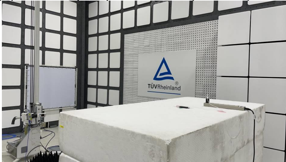
Photograph 5: Test Setup for Spurious Emissions (Back View 4)
