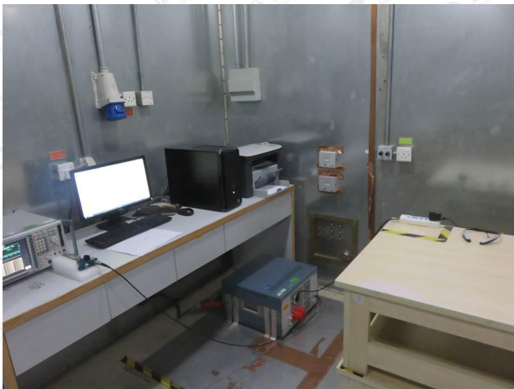
FCC RADIATED EMISSION TEST SETUP
