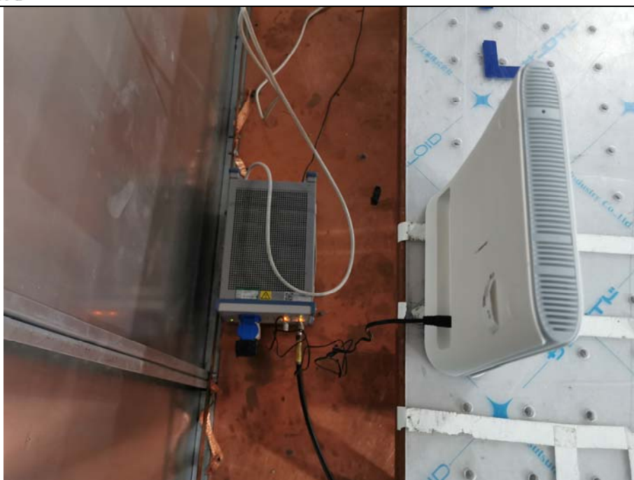
Conducted Emissions Test Setup (with charger)
