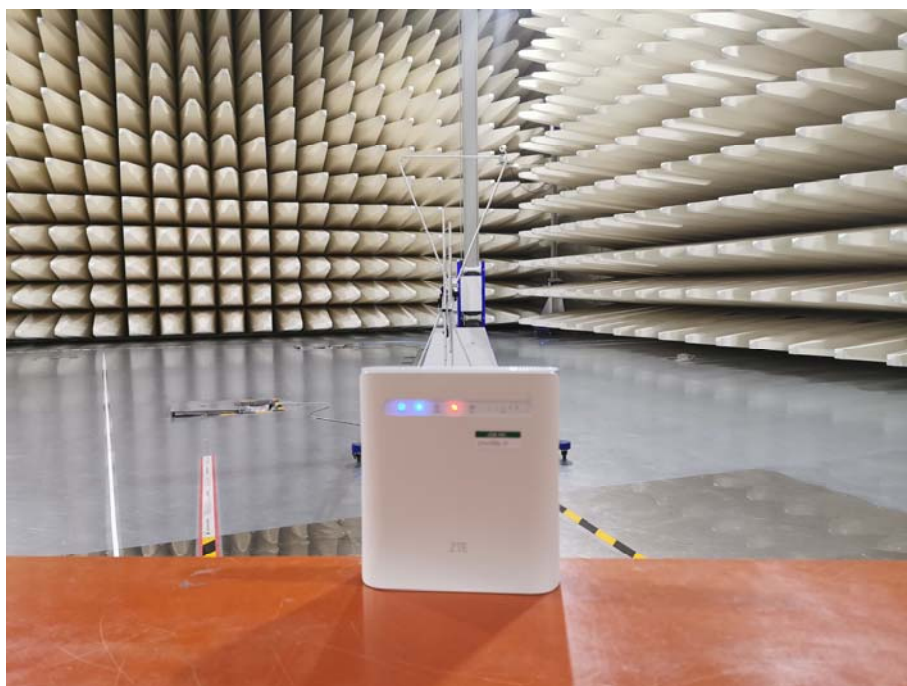
Radiated Emissions Test Setup(below 1GHz)
