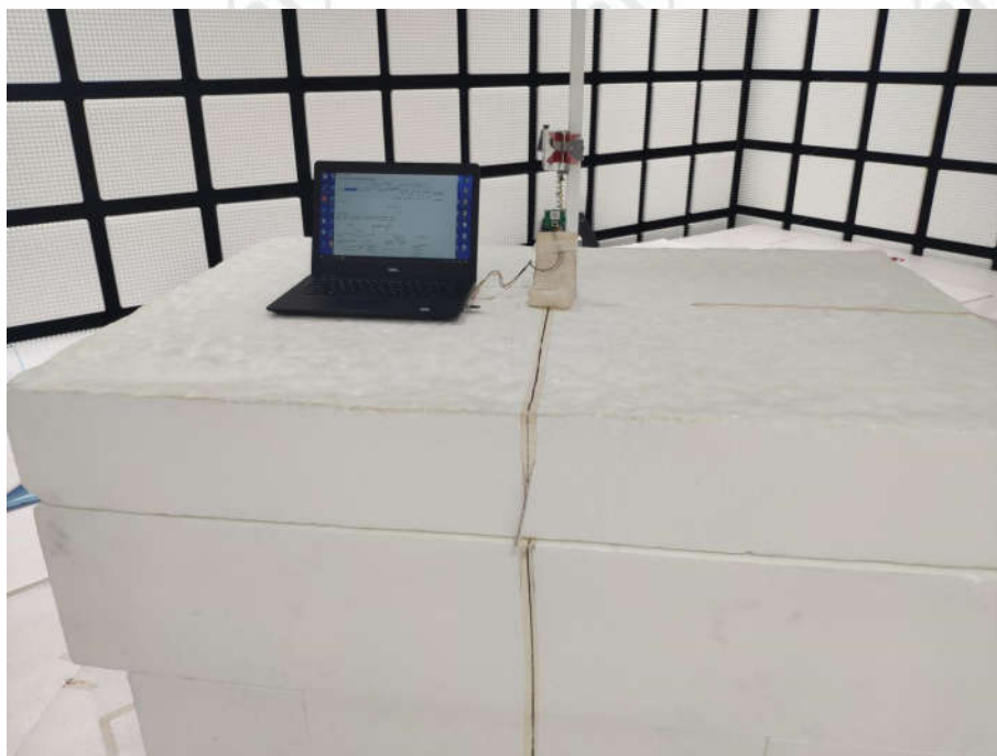
Radiated spurious emission Test Setup-3(Above 1GHz)
