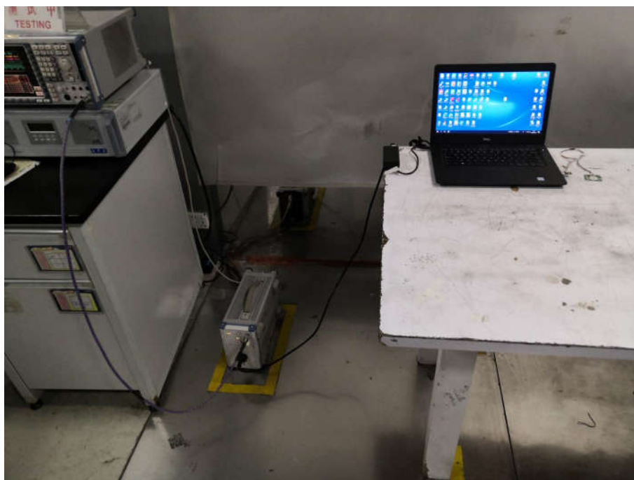
Conducted Emissions Test Setup
