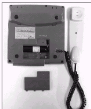
① Remove the back cover of the phone
