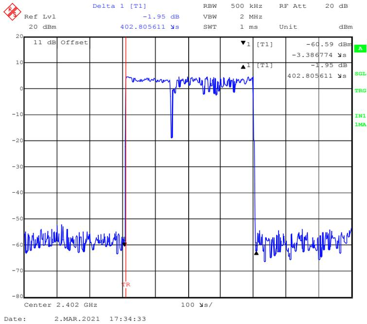
**EDR (8DPSK): Pulse time, Middle Channel, 3DH1**
