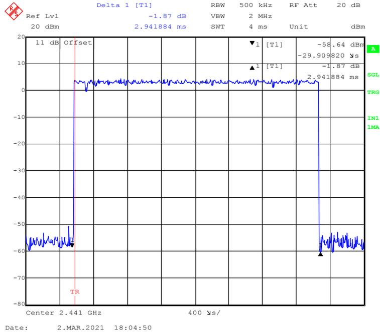
**EDR (8DPSK): Pulse time, High Channel, 3DH5**
