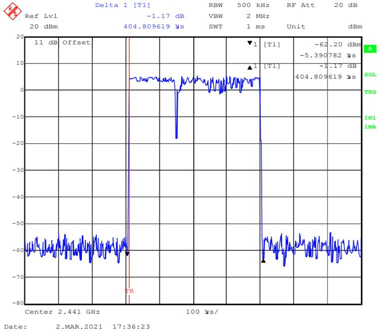
**EDR (8DPSK): Pulse time, High Channel, 3DH1**
