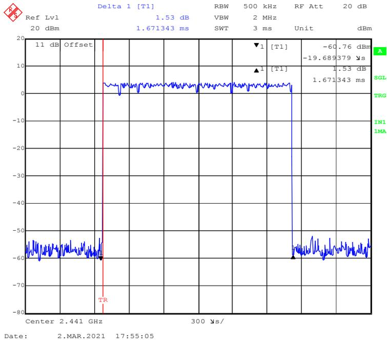
**EDR (8DPSK): Pulse time, High Channel, 3DH3**
