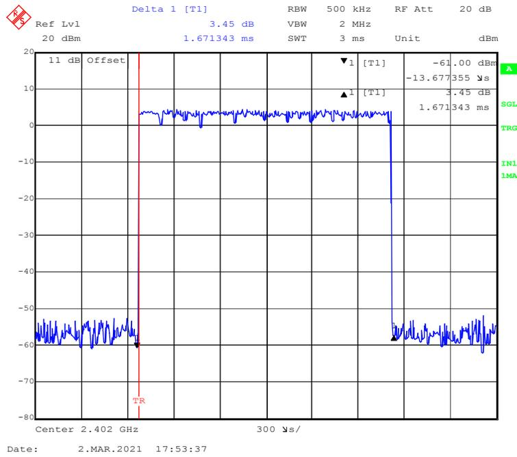
**EDR (8DPSK): Pulse time, Middle Channel, 3DH3**
