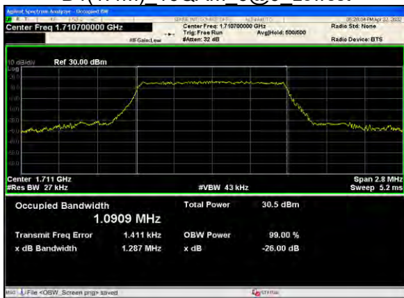
B4(1.4M) 16QAM 6@0 Lowest
