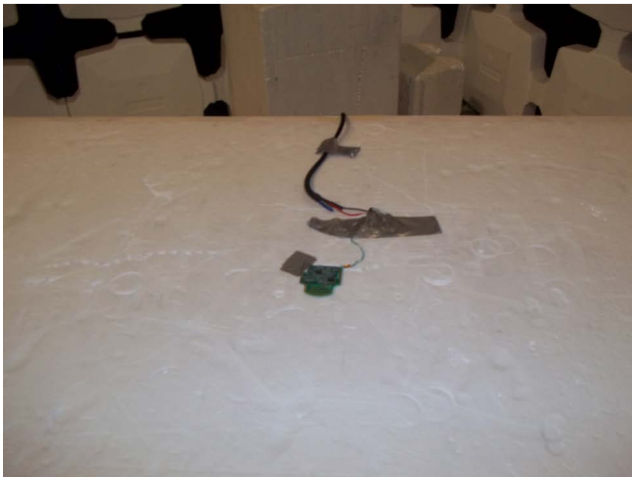
Figure 2. Radiated Emissions Test Setup, UHF (433-435 MHz) Radio
