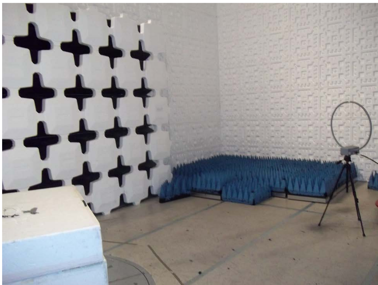
Figure 3. Radiated Emissions Test Setup (9 kHz - 30 MHz)
