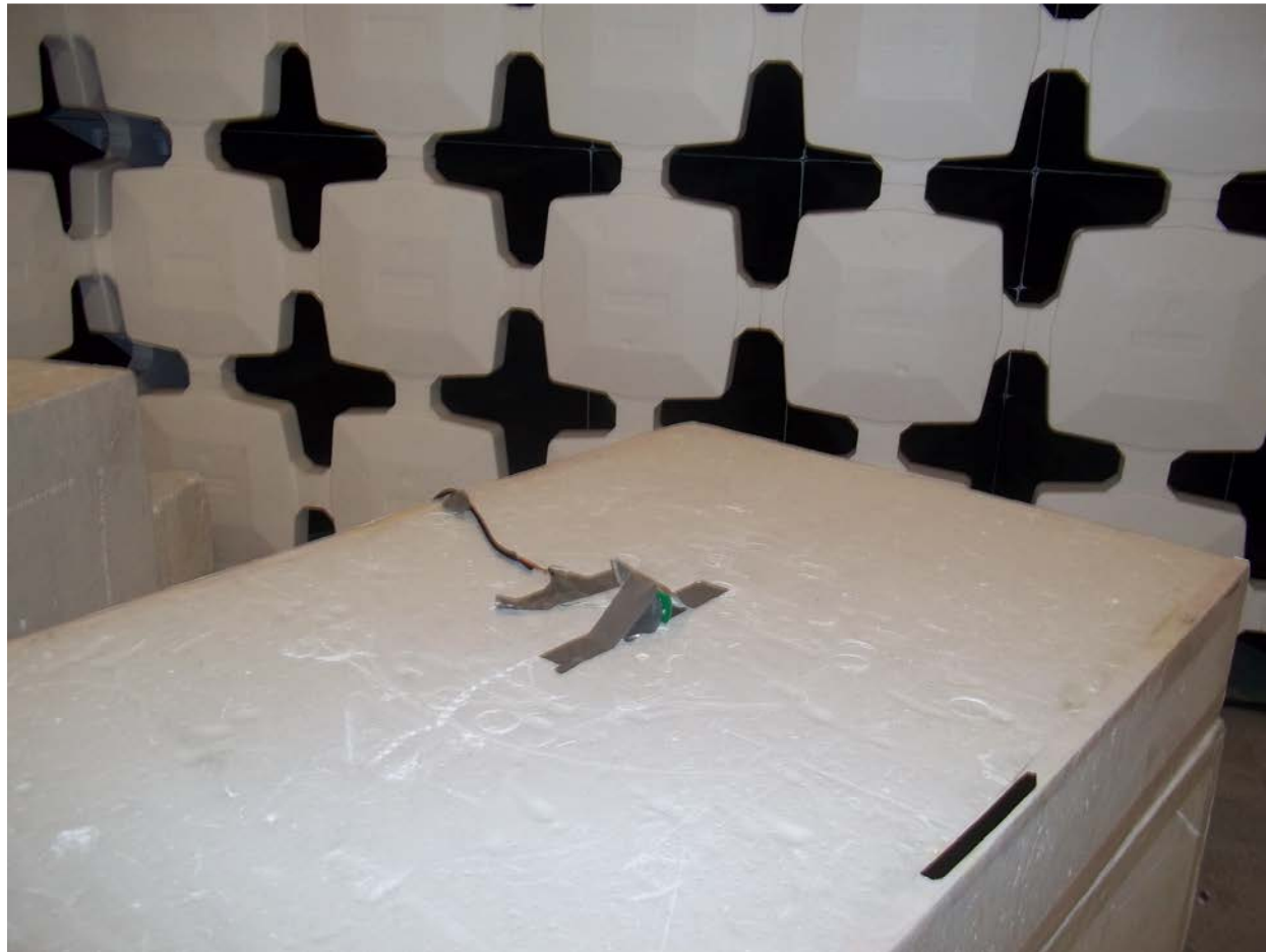
Figure 1. Radiated Emissions Test Setup, BT Radio
