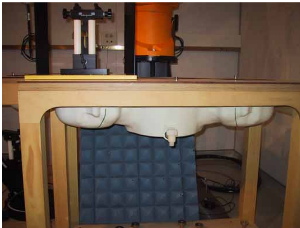
Figure 10.1-1 DASY5 system with absorbing material
