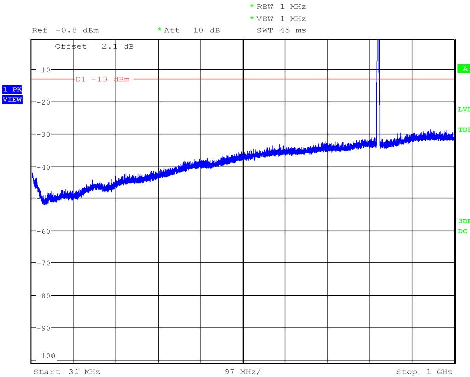
Note: The peak above the limit is the carrier frequency.
