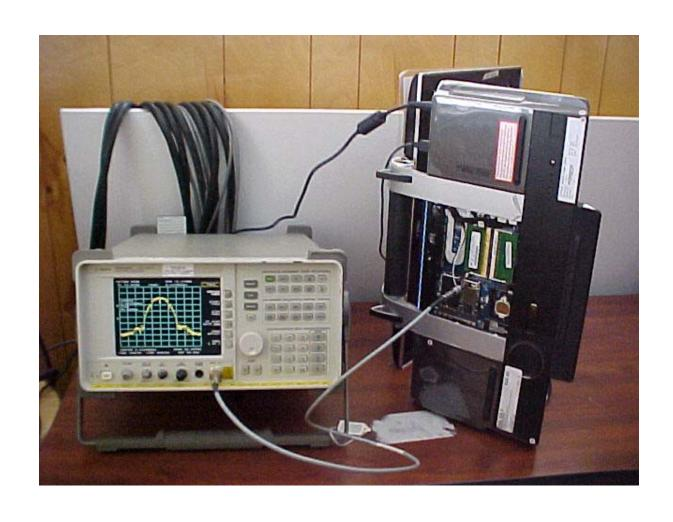
Conducted Emissions at Antenna Terminal Setup
