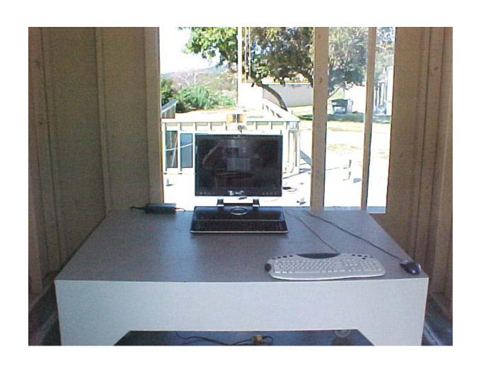
Radiated Emissions Measurement (Front View) Setup
