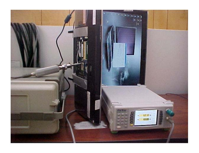
Maximum Peak Output Power Measurement Setup
