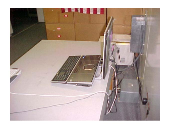
AC Conducted Emissions Measurement (Rear View) Setup
