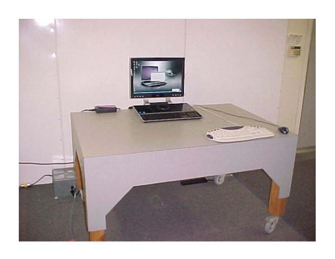
AC Conducted Emissions Measurement (Front View) Setup
