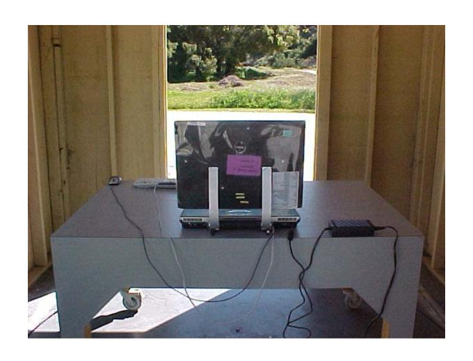
Radiated Emissions Measurement (Rear View) Setup
