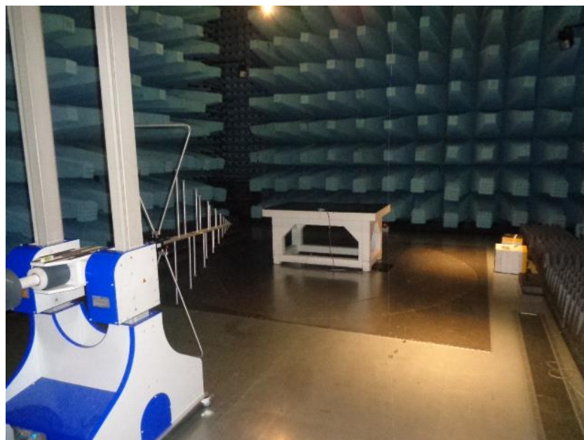
Figure 9.1-2: Radiated emissions set-up for frequencies below 1 GHz
