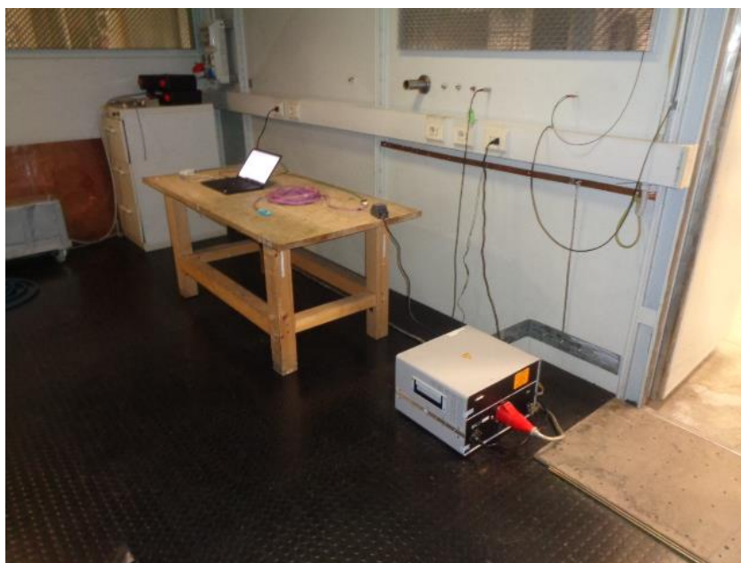
Figure 9.1-4: Conducted emissions set-up
