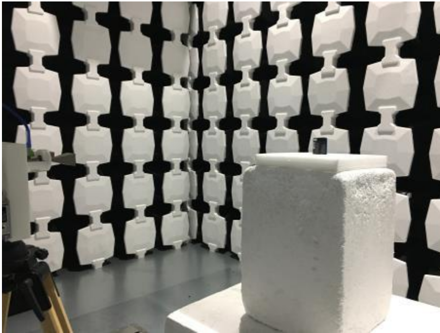
Description: Radiated Emission Test Setup (Above 18GHz)
