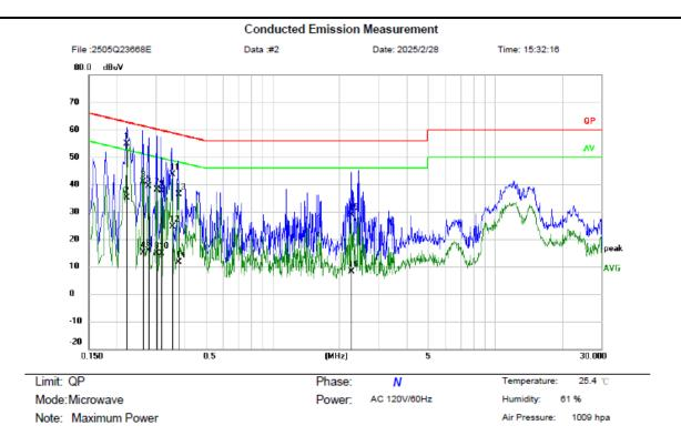
Receiver Setting: 0.15~30MHz: Pre-scan: RBW: 9kHz, DET: PK/AV; Final measure: RBW: 9kHz, DET: QP/AV
