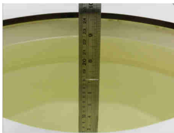
Fig 11.2 Photo of Liquid Height for Body SAR
