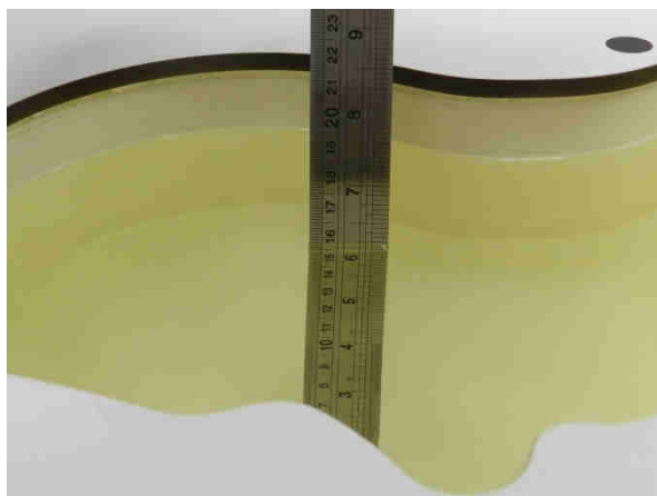
Fig 11.1 Photo of Liquid Height for Head SAR
