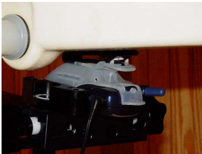
Figure 11.10 body SAR set-up (with holster, slide closed, antenna retracted position)
