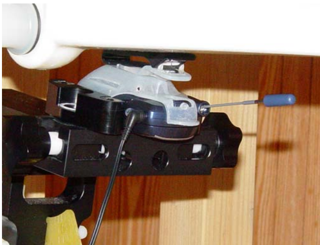
Figure 11.11 body SAR set-up (with holster, slide closed, antenna extended position)
