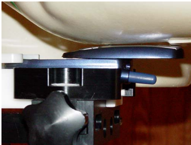
Figure 11.2 phone against the head (left cheek, slide opened, antenna retracted position)
