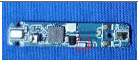
The antenna is Chip antenna.
