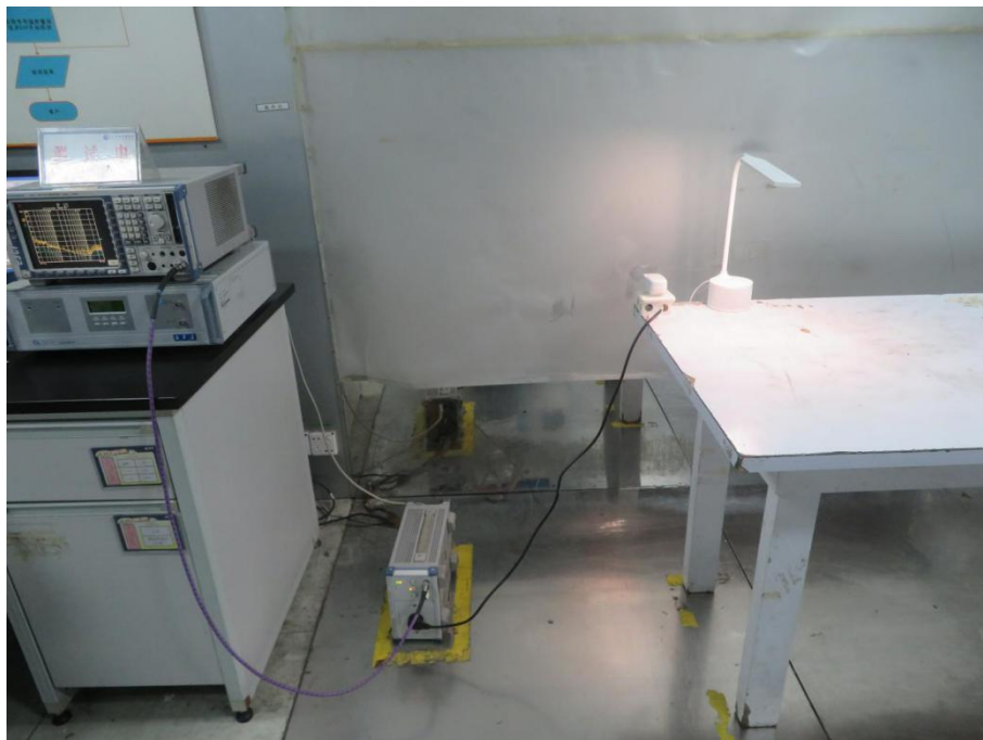
Conducted Emissions Test Setup
