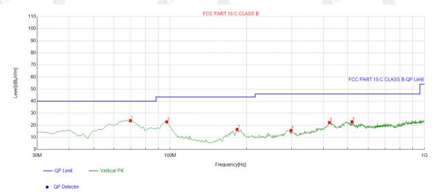
Suspected List Freq. Factor Reading Level Limit Margin Height Angle NO. **Polarity** [MHz] [dB] [dBµV/m]  $[dB\mu V/m]$ [dBµV/m] [dB] [°] [cm] -16.89 40.76 100 69.80981 23.87 40.00 16.13 99 Vertical 2 96.996997 -14.95 37.81 22.86 43.50 20.64 100 194 Vertical 183.41341 -15.63 32.19 16.56 43.50 26.94 100 Vertical 3 79 4 298.95895 -11.75 27.58 15.83 46.00 30.17 100 118 Vertical 423.24324 -8.96 31.26 22.30 46.00 23.70 100 189 Vertical 519.36936 -7.52 30.44 46.00 23.08 100 134 Vertical 22.92
