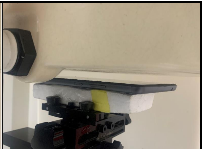
Front Face of EUT with 1.0 cm Gap
