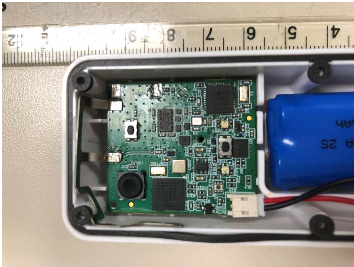
Figure 4 - Parsyl Trek – Closeup of PWB in housing
