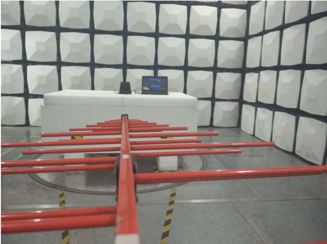
Radiated Emission Above 1GHz front View
