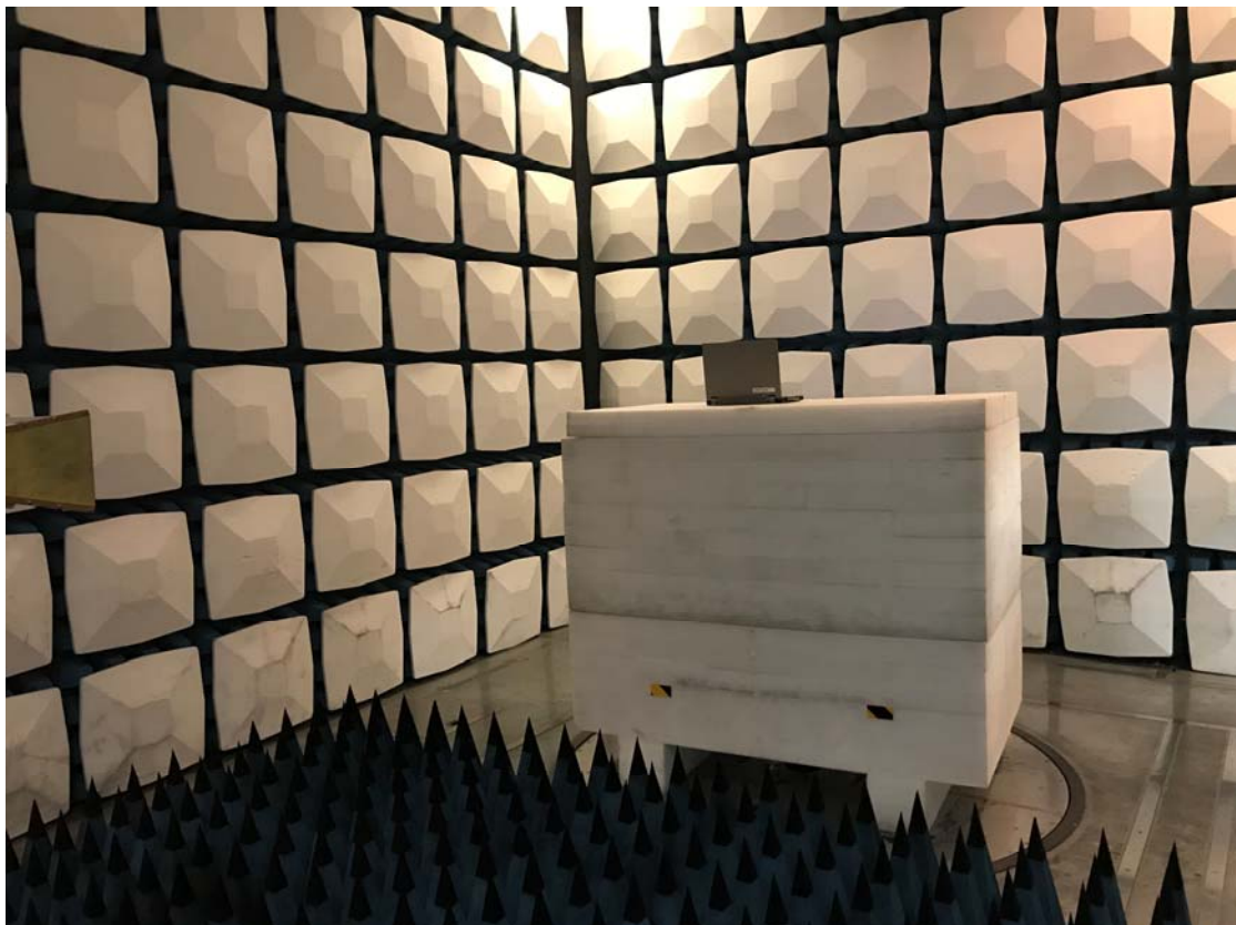
Radiated Emission Above 1GHz front View
