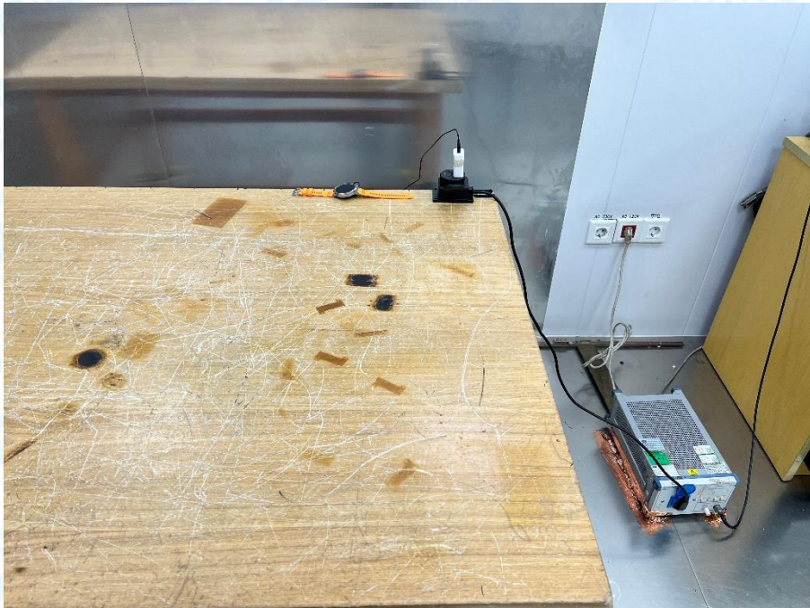
Photo of Setup for Radiated Emission (30MHz~1GHz)
