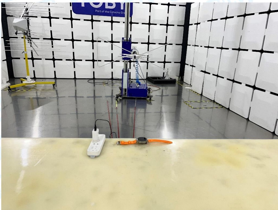
Photo of Setup for Radiated Emission (30MHz~1GHz)
