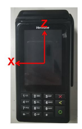
Aux antenna average Gain: -2.8dB Aux antenna peak Gain :1.9dB
