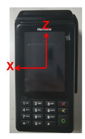
Main antenna average Gain: -2.8dB Main antenna peak Gain :-0.2dB
