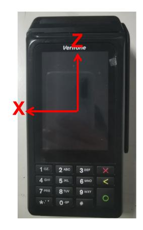
Main antenna average Gain: -6.7dB Main antenna peak Gain :0.2dB
