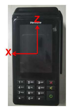
Main antenna average Gain: -3.5dB Main antenna peak Gain :2.7dB
