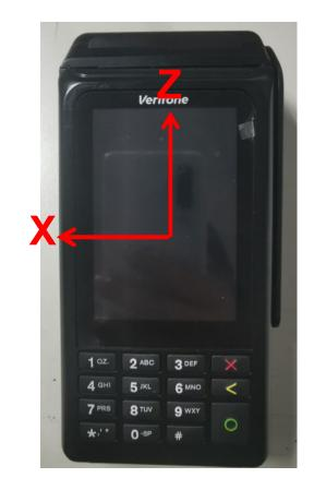
Main antenna average Gain: -3.5dB Main antenna peak Gain :3.2dB
