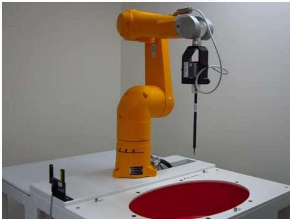
Fig.1 Photograph of the SAR measurement system
