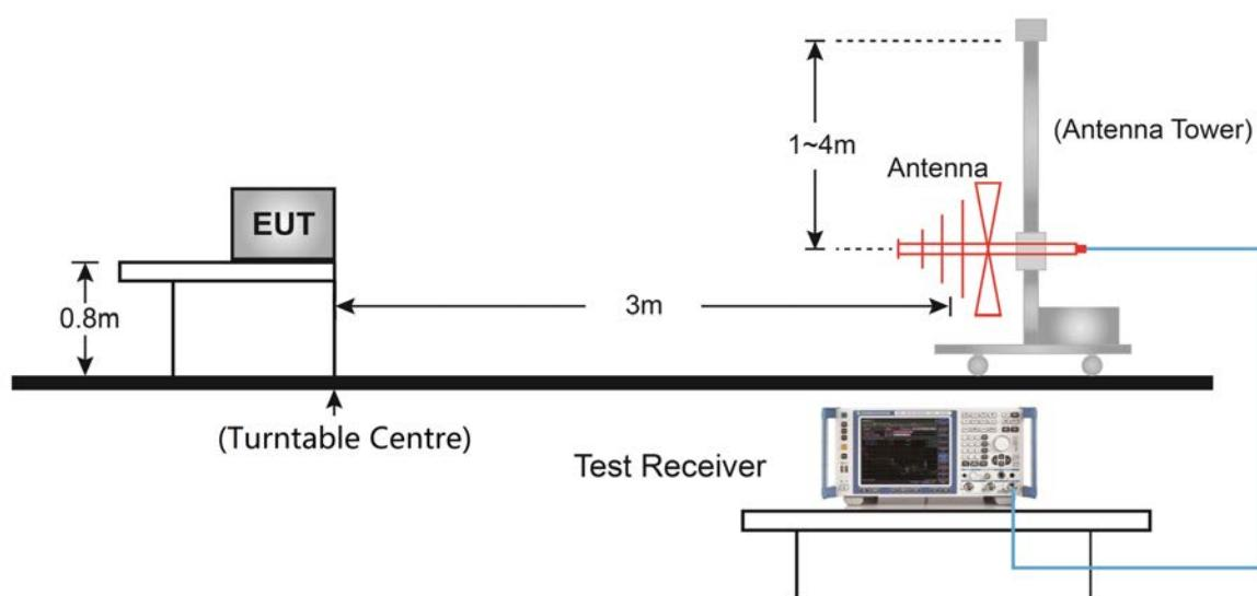
Above 1GHz Test Setup:
