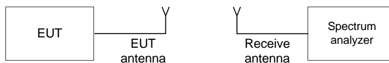
Figure 7.3.1 Hopping frequencies test setup
