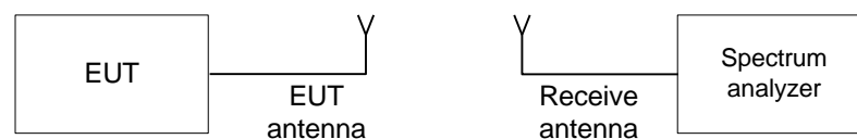
Figure 7.1.1 The 20 dB bandwidth test setup
