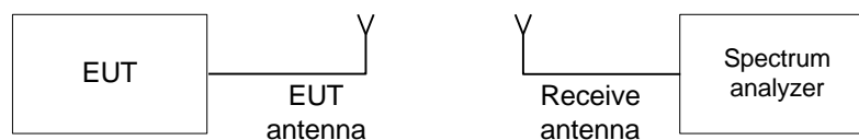
Figure 7.2.1 Carrier frequency separation test setup
