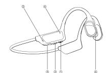
1. Plus kev 2. Substract key 3. Type-C charging port 4 MIC 5 Pilot lamp 6. Horn: bone conduction sound unit
