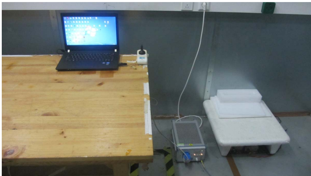
Picture 2 Conducted Emission Test Setup
