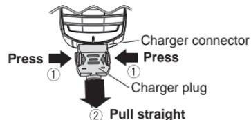
**Make sure to press both buttons and gently pull the charger plug straight.**
