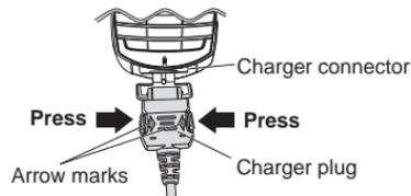
**Make sure to hold the charger plug with the arrow marks facing up and press both buttons.**
