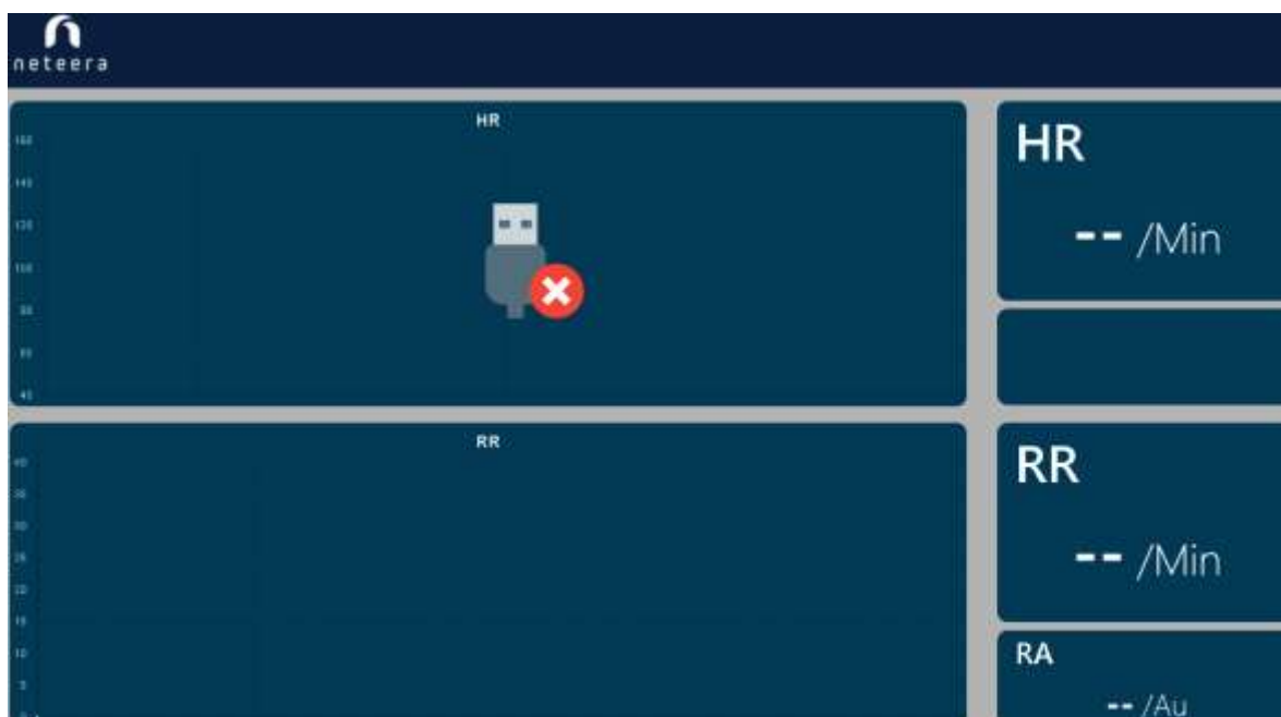
Image 14: – main unit is not connected properly, check the USB cable
