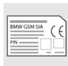
The Bluetooth passkey is located on the back of the snap-in adapter.
