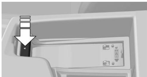
2. Insert snap-in adapter at the front, arrow 1, and press to the bottom, arrow 2, until the adapter engages.
