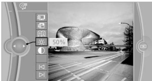
4. Turn the controller until the desired setting is reached and press the controller.
