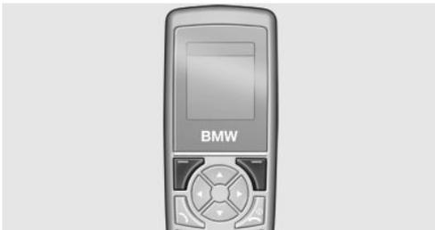
The current functions of these buttons are shown in the bottom line of the display.
