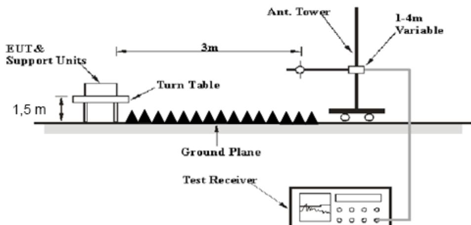
The radiated emission tests were performed in the 3 meters chamber, using the setup accordance with the ANSI C63.10-2013. The specification used was the FCC 15.209, and FCC 15.407 limits.
