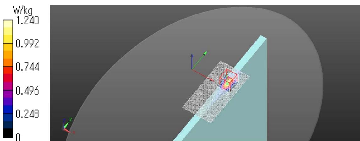
**WLAN 11a 6Mbps Main Ant Edge1 tilt 5805MHz**
