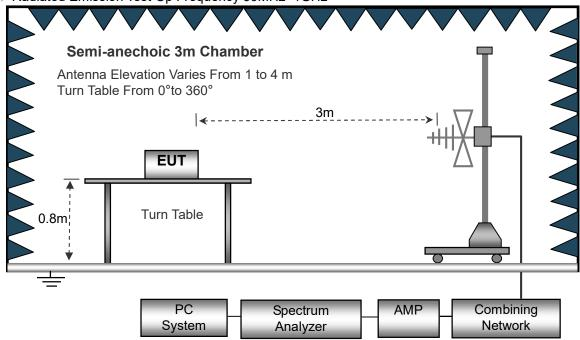
(C) Radiated Emission Test-Up Frequency Above 1GHz
