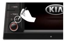
Press the reset hole using a clip or pin.
