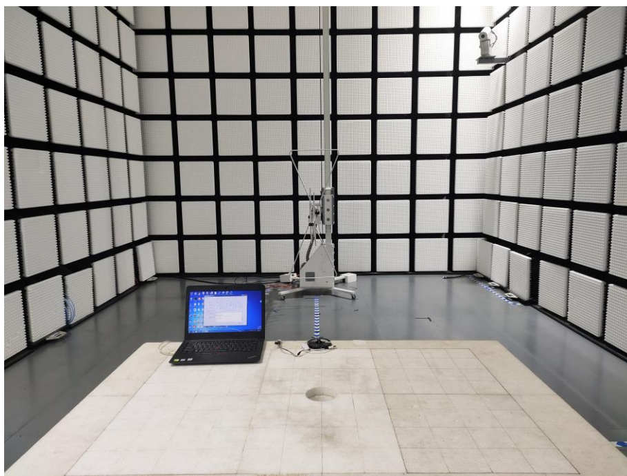
Fig. 2 Radiated emission setup photo(30MHz-1GHz)
