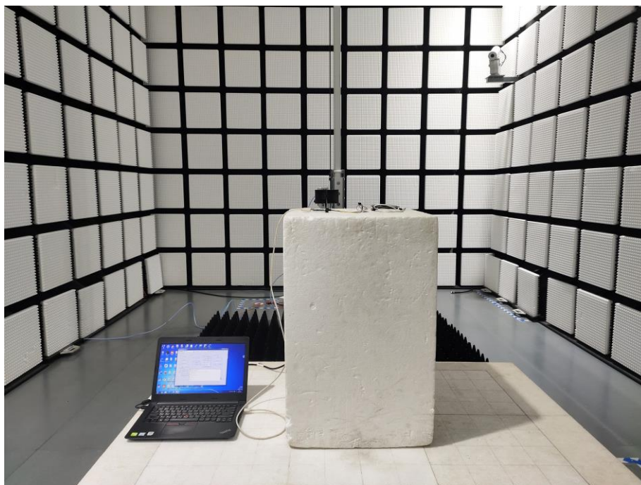
Fig. 3 Radiated emission setup photo(Above 1GHz)
