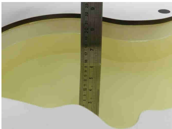
Fig 10.1 Photo of Liquid Height for Head SAR
