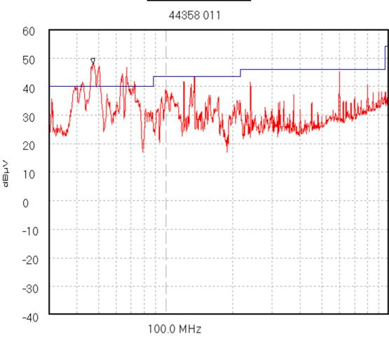
Start 30.0 MHz; Stop 1.0 GHz - Log Scale Ref 60 dBµV; Ref Offset 0.0 dB; 10 dB/div
