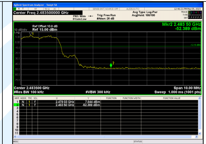
Out Of Band Emission(Right) 8DPSK_3-DH5_Channel Hopping
