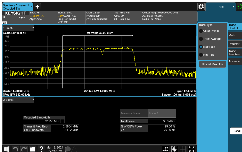
Plot 7-26. Occupied Bandwidth Plot (ULCA LTE Band 48 - 20+15MHz 16-QAM - Full RB Configuration)
