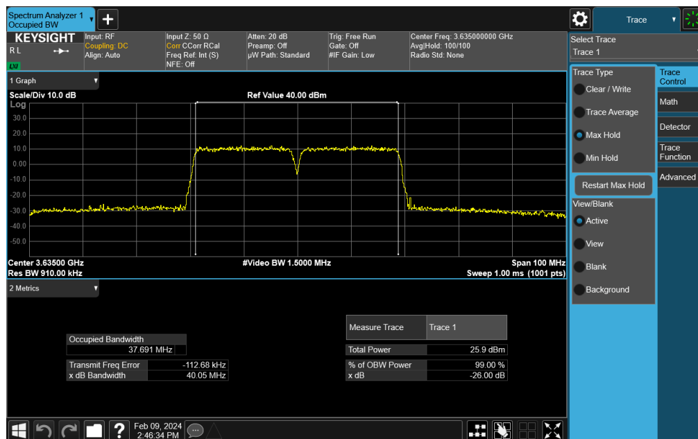
Plot 7-30. Occupied Bandwidth Plot (ULCA LTE Band 48 - 20+20MHz 16-QAM - Full RB Configuration)
