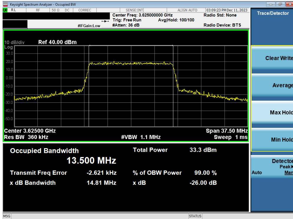
Plot 7-9. Occupied Bandwidth Plot (LTE Band 48 - 15MHz QPSK - Full RB Configuration)
