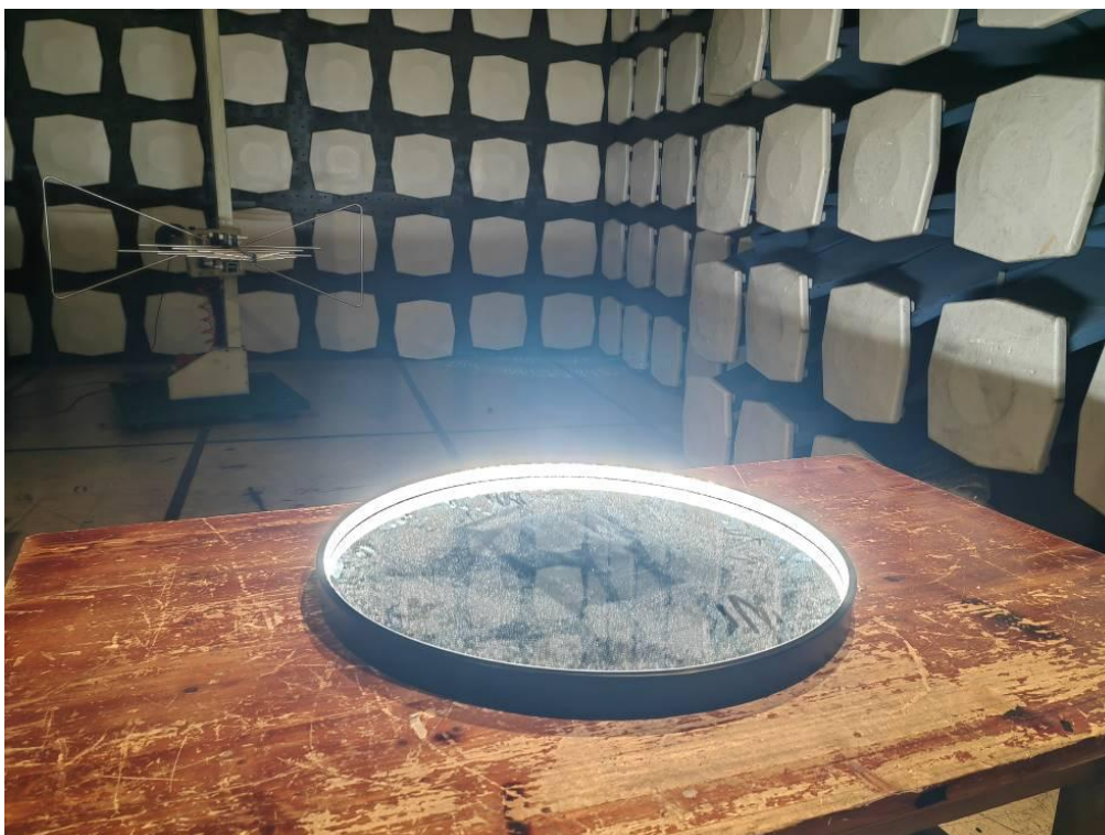
Radiated Emissions, 30MHz to 1GHz Test Setup
