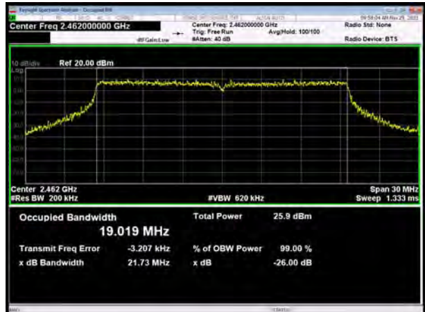
802.11ax(HE40), Carrier frequency (MHz): 2427
