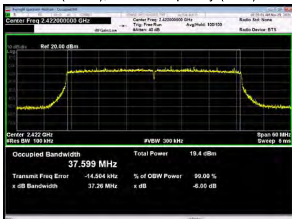
802.11ax(HE40), Carrier frequency (MHz): 2422
