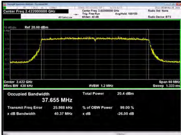
802.11ax(HE40), Carrier frequency (MHz): 2422
