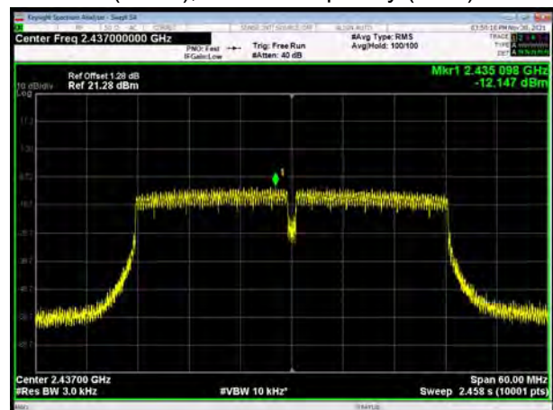
802.11n(HT40), Carrier frequency (MHz): 2437
