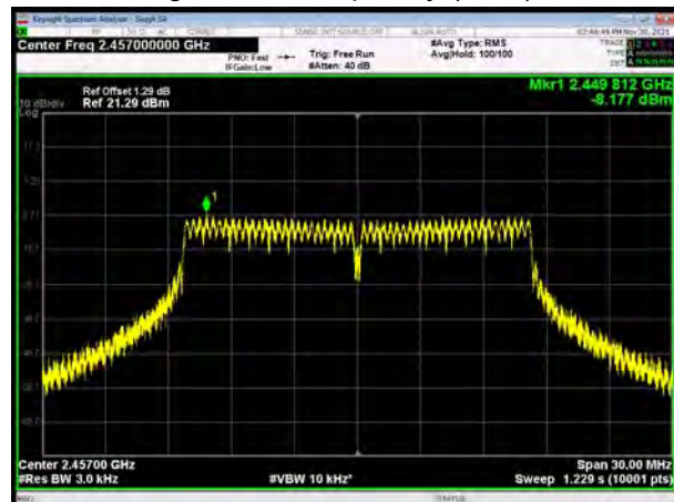
802.11g, Carrier frequency (MHz): 2457
