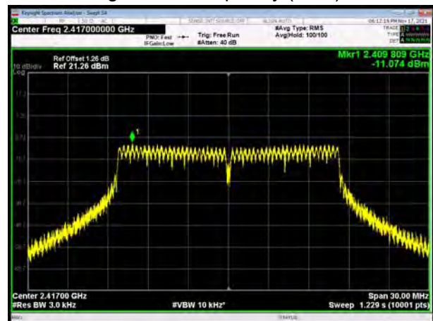
802.11g, Carrier frequency (MHz): 2437
