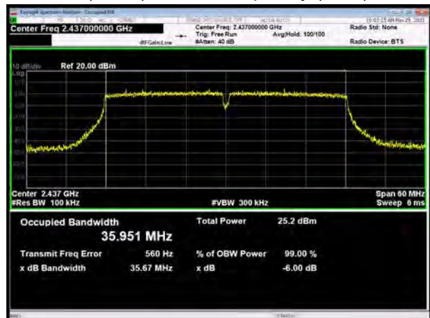
802.11n(HT40), Carrier frequency (MHz): 2437
