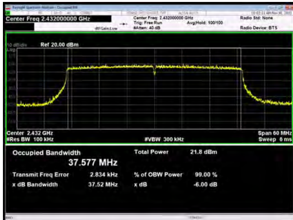
802.11ax(HE40), Carrier frequency (MHz):2442
