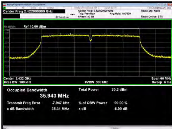
802.11n(HT40), Carrier frequency (MHz): 2432
