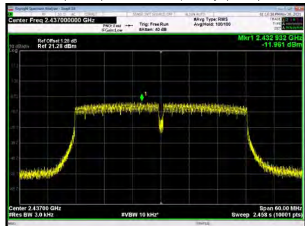
802.11n(HT40), Carrier frequency (MHz): 2437
