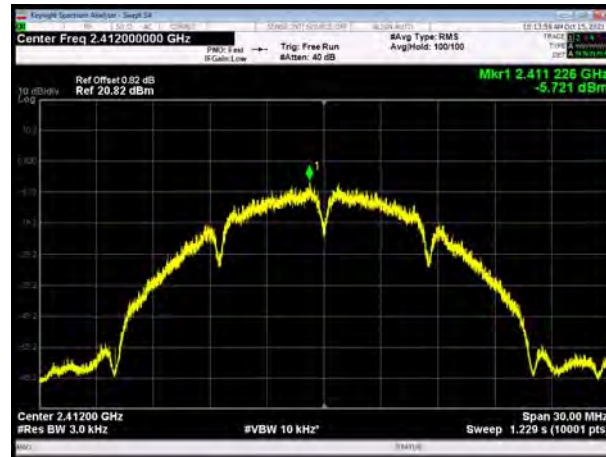
802.11b, Carrier frequency (MHz): 2437
