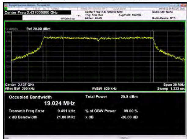
802.11ax(HE20), Carrier frequency (MHz): 2437
